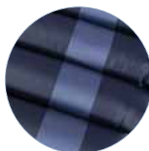
Nylon TPU coated cells
